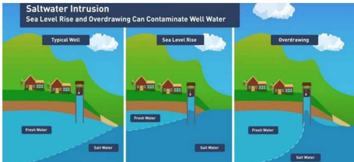
Figure 10: An Illustration Displaying Sources of Saltwater Intrusion into Wells 44
